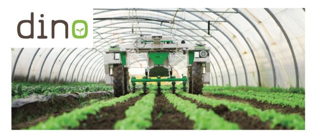
Dino, Naïo Technologies' vegetable bed robot, has officially been released in the field. The robotic straddler weeds vegetable beds to assist produce growers in their daily tasks. Dino guides itself using the same laser and camera system as Naïo's - now famous - Oz robot. It can also use GPS for guidance. The tool is entirely autonomous and works on electrically charged batteries.
