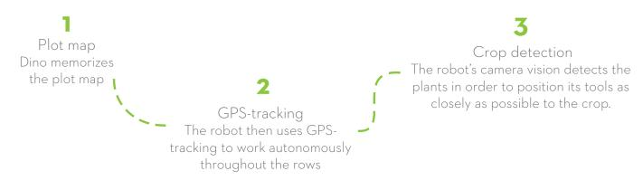
**GPS-guidance** is paired with **camera vision** in order for Dino to be operational in a maximum of configurations while keeping its precision range.
